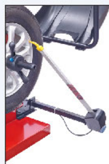
Width gauge measures width of rim automatically 宽度尺
