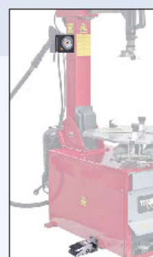
Pedal-controlled inflator 脚踏控制打气表
