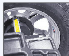
Laser technology for exact detection of tyre and rims defects 激光准确定位轮胎的不平衡位置
